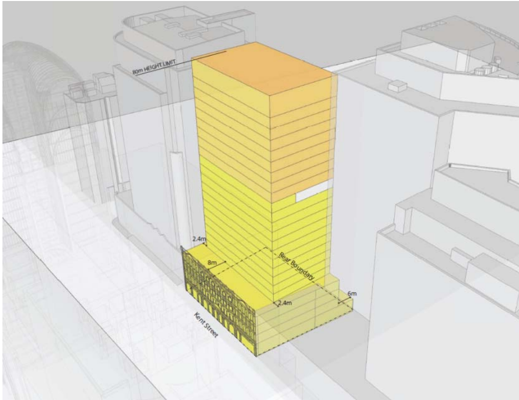
Figure 11: Proposed building envelope looking south
